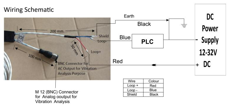
The machine/ surface on which the sensor is mounted, must be 'earthed' properly. It is recommended to connect the -ve terminal of voltage to earth potential to minimize interference.
